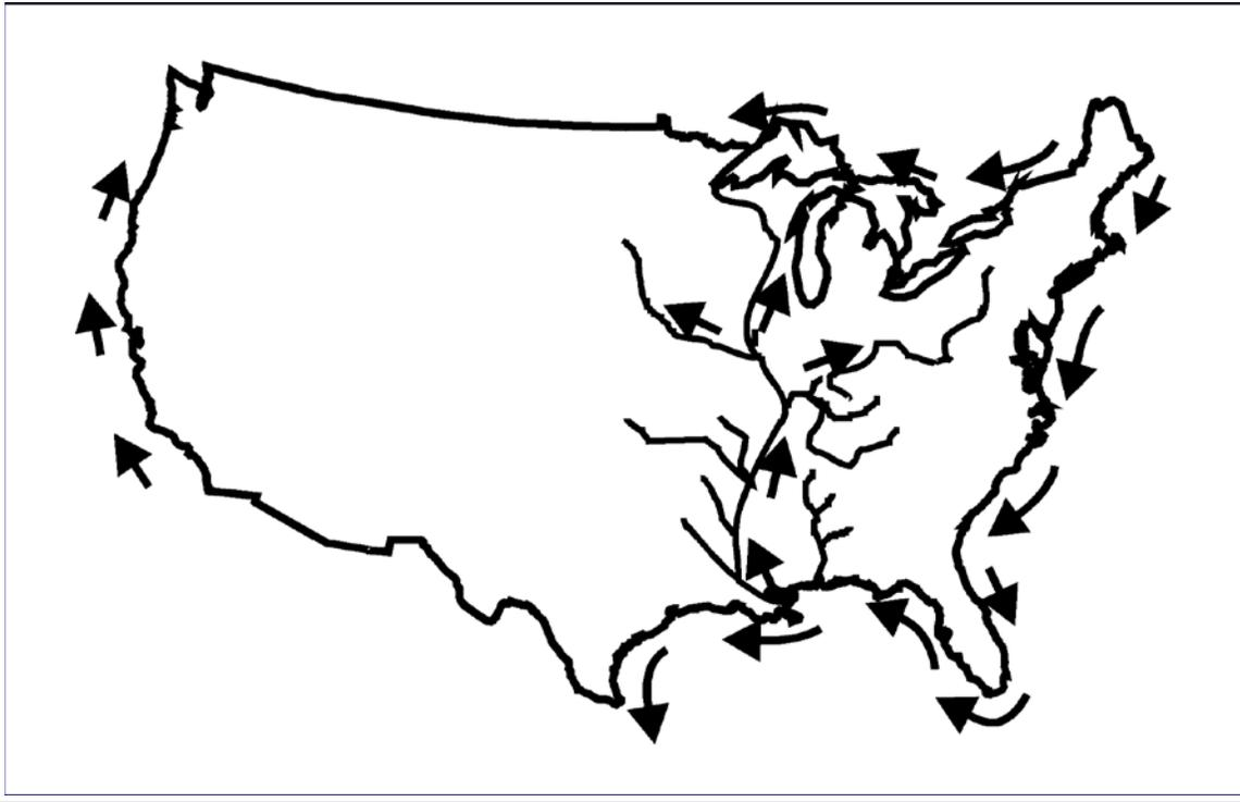
Figure 2 – CDB - Conventional Direction of Buoyage Graphic
